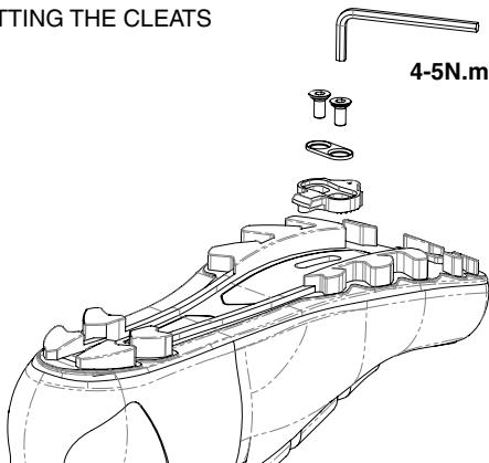
Make sure that the sole is clean where it meets the cleat, and clean it with a damp cloth if necessary. Lubricate the screws and tighten them to a torque of 4 to 5 N m using a high-quality 4 mm Allen key.
