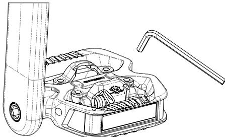
The pedals cannot be adjusted while the cleats are clipped in. You will know that you are approaching the maximum setting when it becomes harder to turn the screw. Once you reach this point, stop turning the screw to avoid damaging the pedal.
