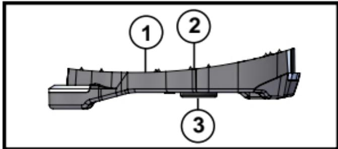
**2: Axle - pedal marker:** this mark corresponds to the position of the axle of the pedal when the shim is engaged in it.
