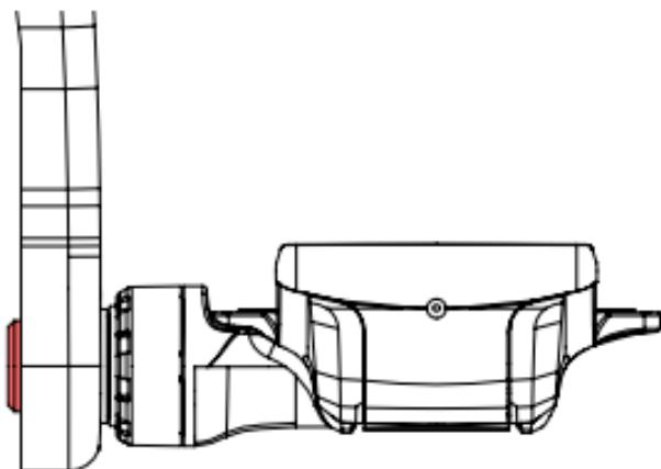
**4 : PAD:** Play adjusting pad to be inserted between the cleat and the pedal, and essential for correct operation.
