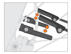
The ESC-system prevents locking of the front wheel when a foreign body should be caught between tyre and mudguard. The stays release in such a case automatically. These can be pressed in again afterwards.
