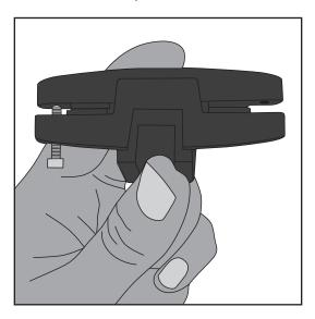
2. Attach the click system to the rear of the saddle and mount it.
