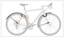
**EN** . Mounting rubber inlays & Fastening with velcro and rubber straps
